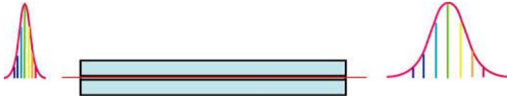
Figure 2 – The effects of dispersion on a light pulse
